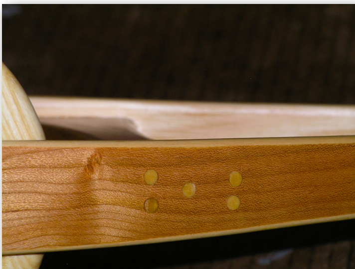
Pictures showing other joinery techniques; Dowels in my Clacker and Dovetails in my Block Wagon.
