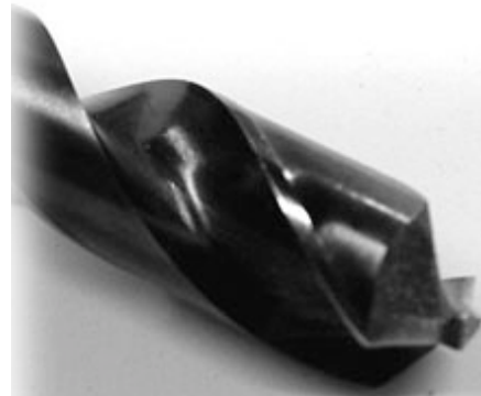
My letter size V bit reground with a Krenov pilot.
